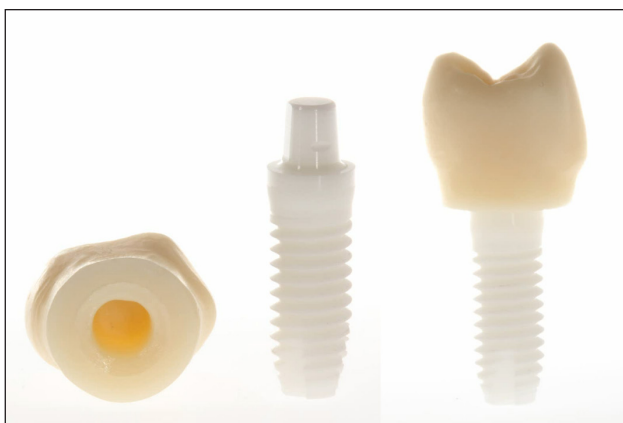
Fig 1 Ceramic crown and one-piece zirconia implant. The ceramic crown was deliberately overcontoured (1.5–2 mm) in the marginal area to prevent the assembled implant-crown complex from sliding out of the test fixture during the debonding process in the universal testing machine.
