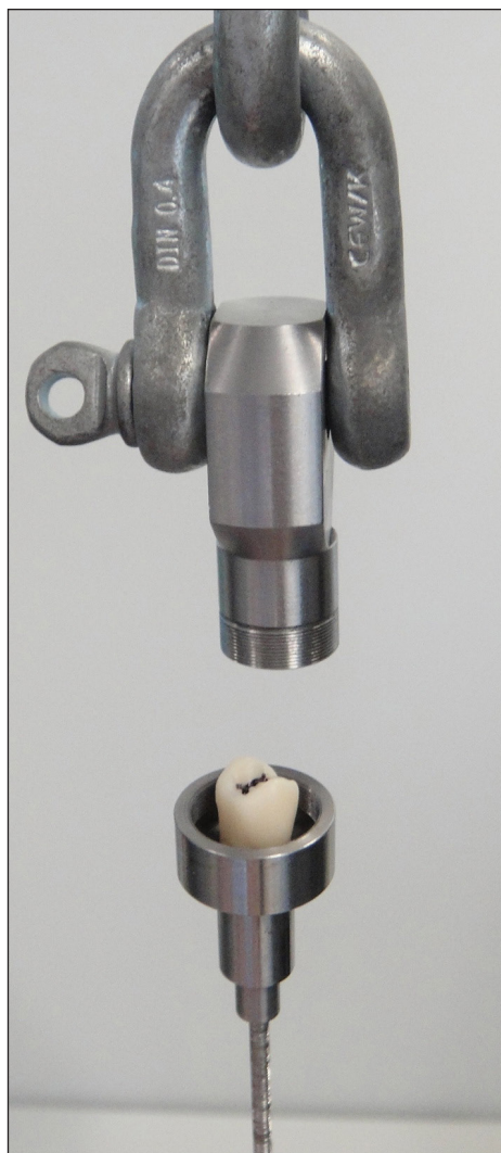
Fig 2 Specimen fixed to the lower mounting box of the universal testing machine.
